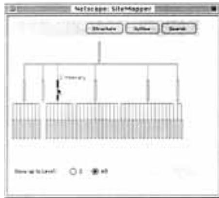
Figure 4-16. In this example of an automatically generated site map, go bars represent pages within a web site. Users must roll their cursor over a Solid bar to see the title of the page. Do you think this approach is more useful than a text-based table of contents?
